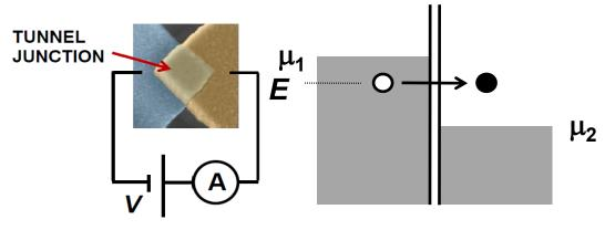
Dissipation generated by a tunneling event in a junction biased at voltage V
